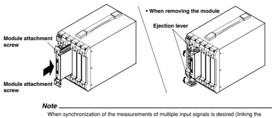
modules), install the multiple digital thermometer modules in adjacent slots.
