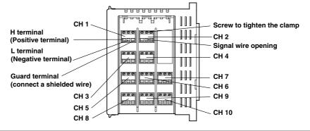
When connecting the input signal wire to the clamp type terminal, loosen the screw holding down the clamp, insert the input signal wire into the opening, and then tighten the screw.
