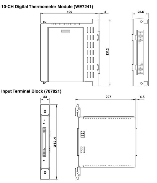
If not specified, the tolerance is  $\pm 3\%$ . However, in cases of less than 10 mm, the tolerance is  $\pm 0.3$  mm.
