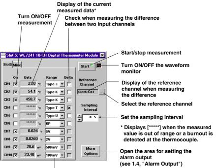
Select the thermocouple type/measurement range
